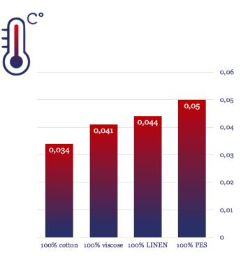
Insulation / Thermal Resistance Rct- m2 k/W Skin Model ISO 11092 standard
