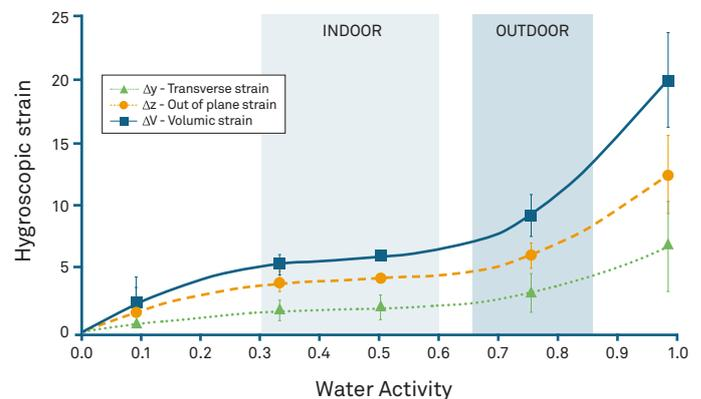
Figure 2: Figure adapted from Réquillé et al. [7], hygroscopic strain (%) in unidirectional hemp fibre reinforced epoxy composites conditioned until saturation in function of water activity. The indoor area ranges from the average relative humidity in winter to the summer average in residential buildings in Western Europe. The outdoor area ranges from the average relative humidity in summer to the winter average in the Western European outdoor climate.
